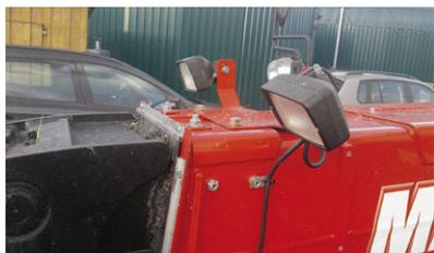
Working lights on the telescope
