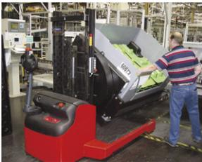
Electrical pallet truck with rotator
