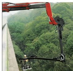
MRT with 3D system to work under the zero level
