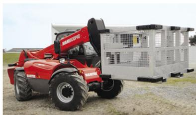
MHT with a 1200 kg capacity mine platform
