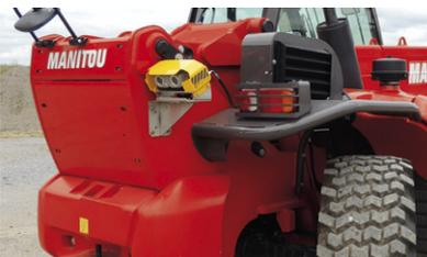
On-board camera for pedestrian detection, alarm and warning light in the cab
