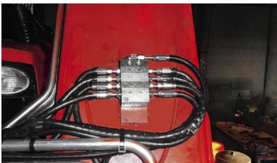
Centralised lubrication at the foot of the boom
