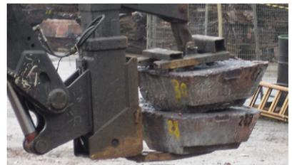
Attachment adapted for pig copper handling\*
