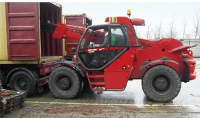
MHT: unloading of a 20 feet container
