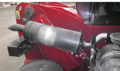
*Exhaust, catalytic converter, fire screen*
