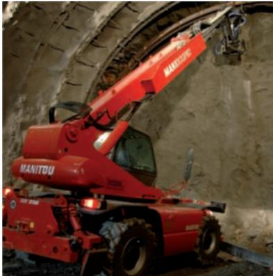
MRT 2150 with 4t (8820lbs) capacity Rib Erector
