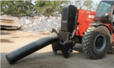
MHT 10180 with 10t (22046lbs) capacity spike
