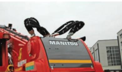
Reinforced synthetic fiber sleeves to protect the hoses
