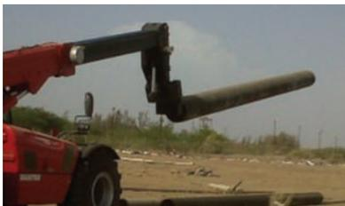
MHT 10210 handling a 12m (470"), 2,200kg (4850lbs) pipe with a prong
