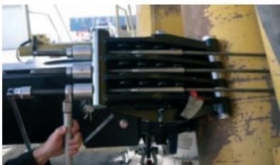
CH4 clamping torque controller
