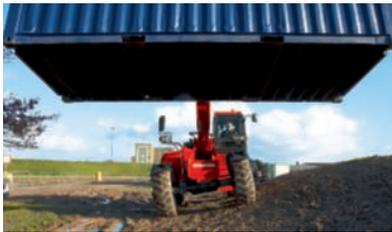
MHT rough terrain handling with levelling correction
