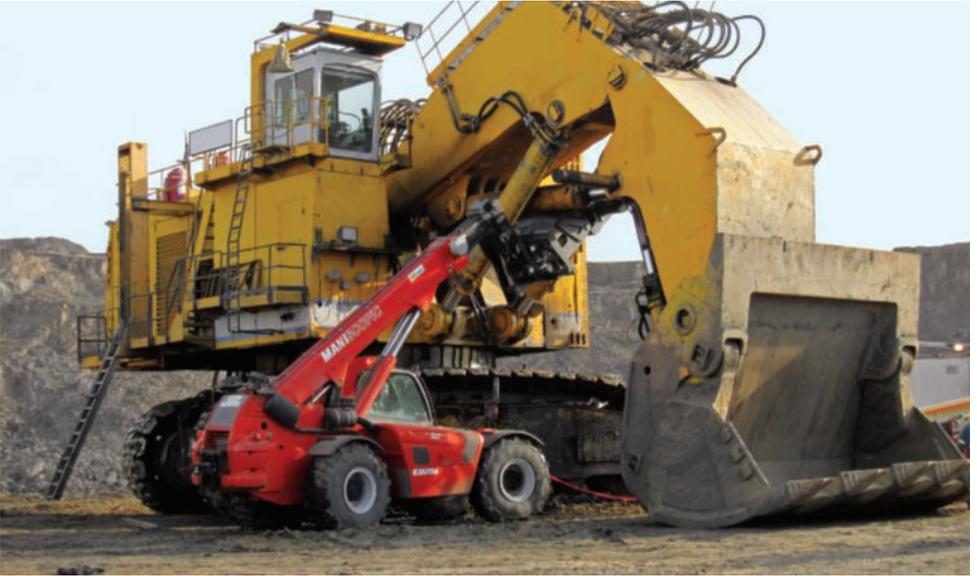
MHT 10160 + CH10 servicing a 9,80 ton (21605lbs) excavator
