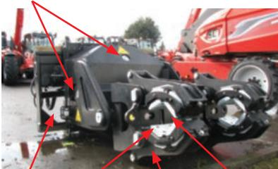
Warning lights    Reduction pads    Pad shoe    Accumulator
