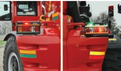
Signal lights for machine approach or withdrawal
